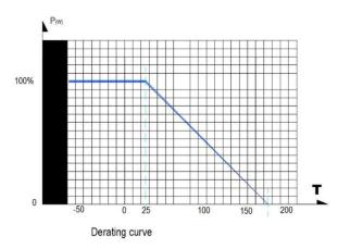
This value is only valid by using a thermal conduction to the heat sink Rth-cs<0.025°K/W.
